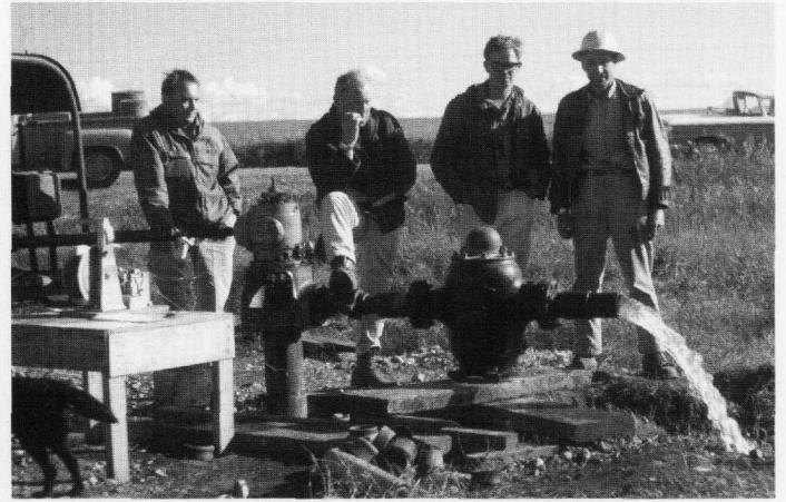
Figure 3. Testing a successful well, sited on the basis of flow-system theory, Olds, Alberta, 1964 (J. Tóth standing far left).
